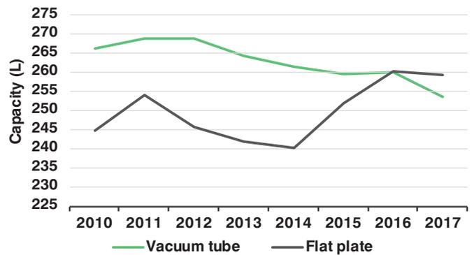
Figure 19 shows that large-scale FP SWH systems are normally bigger in area than large-scale VT SWH systems. Figure 20 shows that large-scale FP SWH systems also have a higher average capacity (in liters) than VT systems. Due to few installations of large-scale systems, evident fluctuations can be seen within the graph. Large-scale systems have an overall average area of around 35 m<sup>2</sup>/system and a capacity of around 2,000 L/system.
